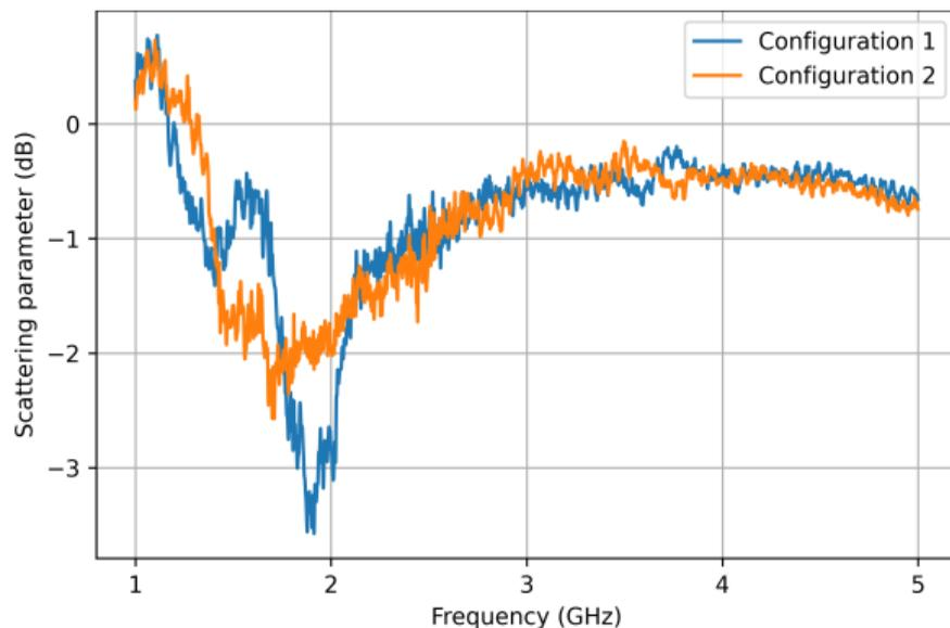
Figure: The configurations are two parallel 4 cm wires with different separations between them.
