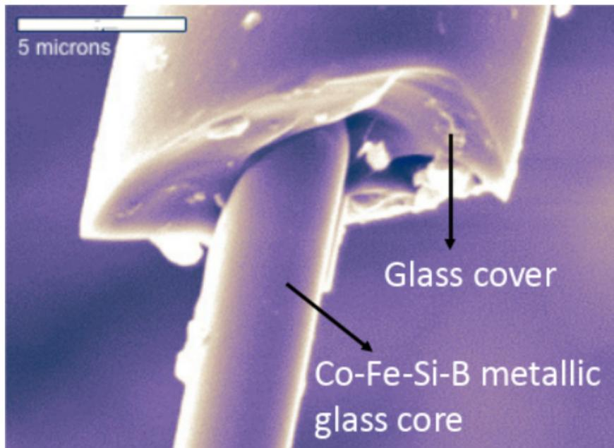
Figure: SEM micrograph of glass-coated microwire.<sup>a</sup>
