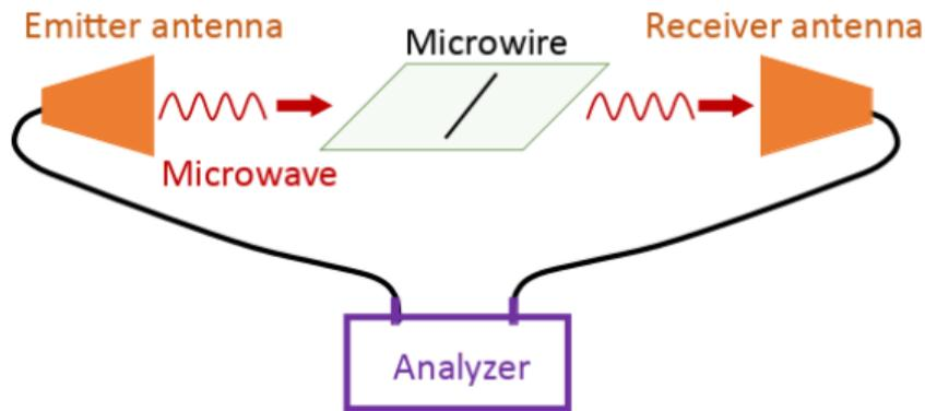
Figure: Schematic of experimental apparatus to measure the  $S_{21}$  response of arrays of MWs.
